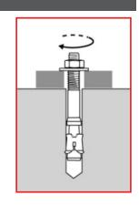
4. With correct size socket tighten anchor to the specified torque
