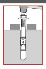
3. Install anchor through fixture into position
