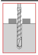
1. Drill hole with correct drill bit to the correct hole depth
